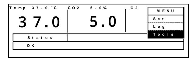
**2.** Select *Date Time* from the Select Tools Display, press the MENU Key to display the menu, select *OK*, and press the ENTER Key.
